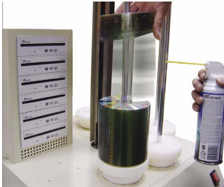
Figure 1-1 Using Canned Air to Reduce Static
